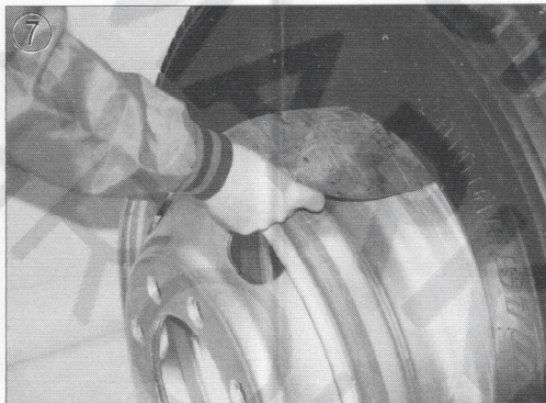
7 Stand the tire up and slide the inner tube between the wheel and the tire.
