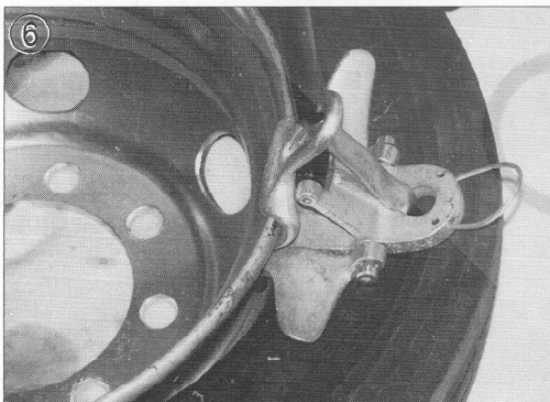
After the spoon tip is in the hole on the clevis, give the lever one last push to make sure the clevis is set completely into the drop center.
