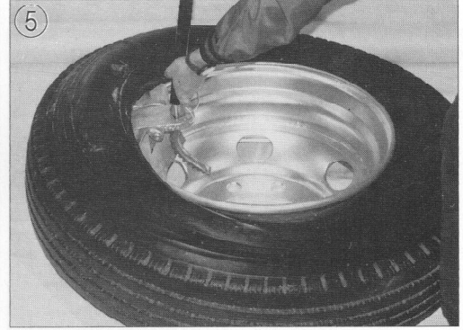
5 After reinserting the crook end, grip the wire of the clevis and the base of lever bar with one hand.
