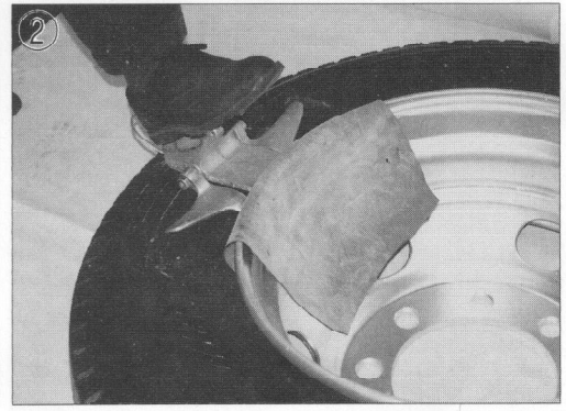
2 Place the clevis behind the inner tube and push down with foot.
