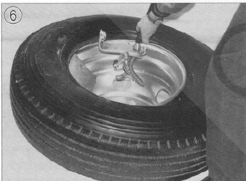
6 While keeping one hand on this assembly, dismount the tire with the other hand and take the clevis and lever bar out of the center of the tire as one piece. This technique prevents the clevis from falling into the drop center and scratching the wheel.
