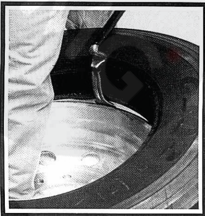
Step 1: Place the lip of the J1 on the flange of the wheel and force the first bead of the tire downward.
